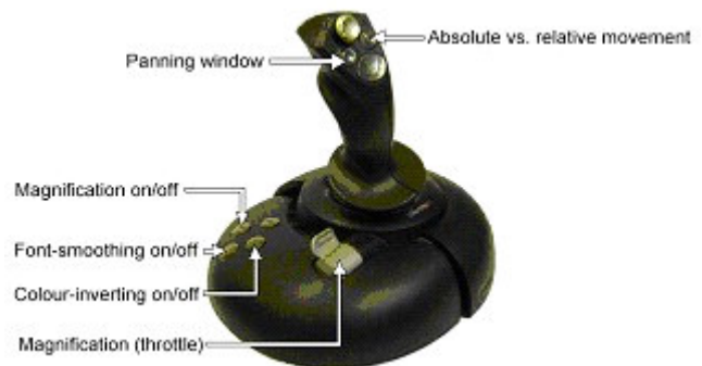
Fig. 2. The mapping of control buttons to magnifier features in the first tested joystick.
