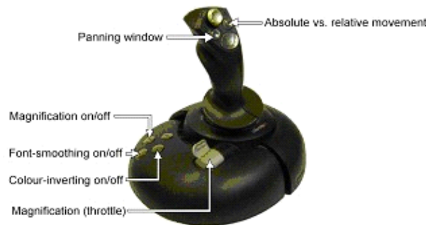
Fig.9. The mapping of buttons to magnifier features in the joystick used in the first study (taken from [8]).
